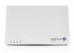
Unique in the industry, the compact OmniAccess 203R remote AP is software configurable to operate in either 1x1 dual radio mode, or 2x2 single radio mode. It supports up to 867Mbps in the 5GHz band or up to 400Mbps in the 2.4 GHz band when operating in single radio 2x2 mode. In dual radio 1x1 mode, the maximum data rates for the 203R AP are 433Mbps in the 5GHz band and 200Mbps in the 2.4GHz band.
